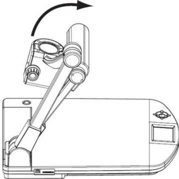
4. Move the lamp column and the lamp head to an appropriate position.
