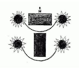
Figure 6.1. East-west orientation of the home. With the long axis built as above, the smaller sides of the home receive less hot summer sun than the long walls would if oriented differently.
