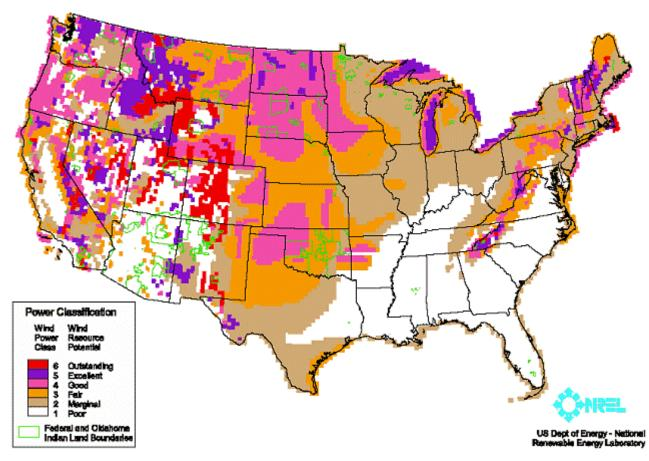
Figure 2.2. Map of Wind Potential in United States. This map is reproduced from the Energy Information Administration website and shows the wind potential in the contiguous United States. Most of central Maryland shows a poor rating with a fair to possibly good rating in the western portions and the eastern shore of Maryland.
