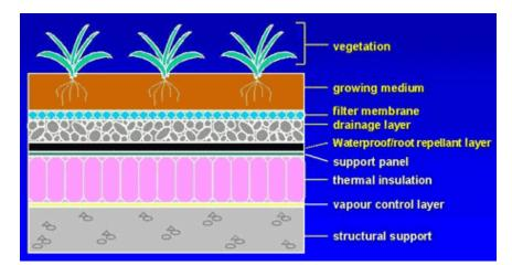
Figure 6.4. The layers of a general green roof and how they are arranged.
