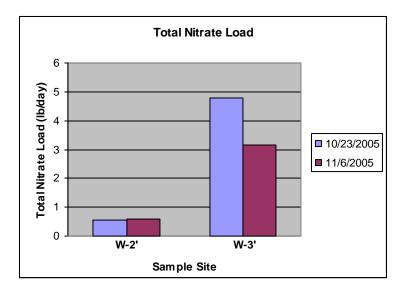
**Figure IV-10.** The total nitrate load into Norris Run on two different days. The first site is just downstream from interstate 795 (W-2'), and the second site is slightly downstream from the farm (W-3').
