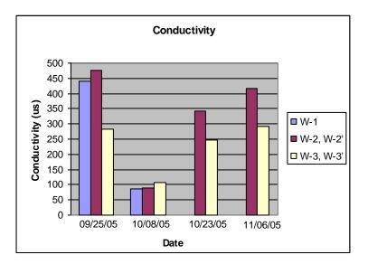
**Figure IV-9.** The conductivity of Norris Run on four different days at three sampling sites, near the beginning of the stream (W-1) after it passes under interstate 795 (W-2) and as it flows by the farm (W-3). The weather had been extraordinarily dry in September but the drought broke on October 8.
